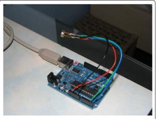
Figure 9 The infrared sensor being tested on an Arduino circuit board.
